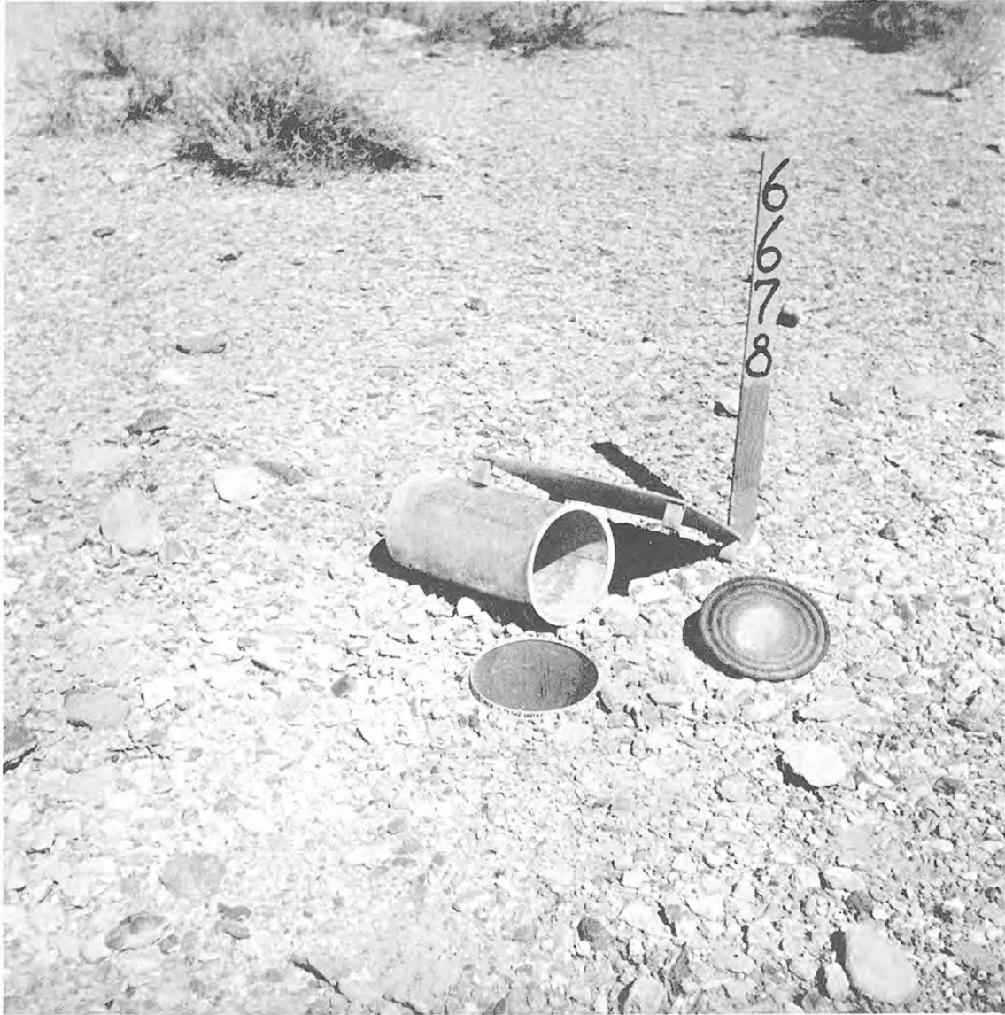
Figure 4. Can trap, trap insert, lid and cover. To the right is a sample stake.
