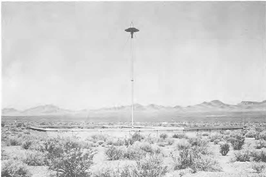
Figure 2b. Radiation source atop a 50 ft tower. The source is shielded to create a relatively uniform radiation field.
