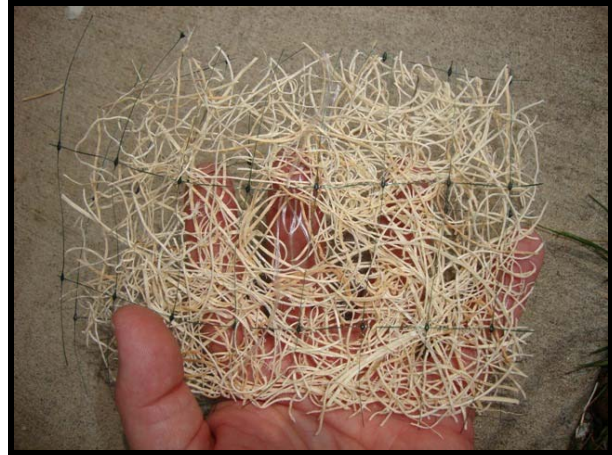
FIGURE 2. Example of an erosion control blanket (ECB) product that incorporates biodegradable woodstraw and two layers of a synthetic polymer mesh (note elongated apertures). (Photograph of a manufacturer's sample square by Josh Kapfer)
