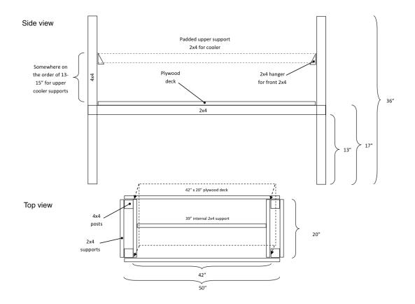
Appendix 1. Side and top view schematics for wooden cooler cradles with supplies and appropriate dimensions (see text for metric measurements) of a Hellbender (*Cryptobranchus alleganiensis*) transport system.
