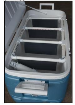
FIGURE 2. An interior view of a Hellbender (Cryptobranchus alleganiensis) holding cooler with plastic baffles, outflow PVC elbow and pipe, and attached drainage grate. (Photographed by Brian Tornabene).
