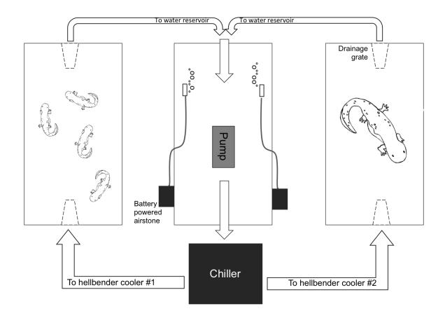
**APPENDIX 2.** An illustrated depiction of water movement through the Hellbender (*Cryptobranchus alleganiensis*) transport system and its working parts ( $1.3 \times 1.5 \text{ m LW}$ ,  $50 \times 60 \text{ in. LW}$ ).
